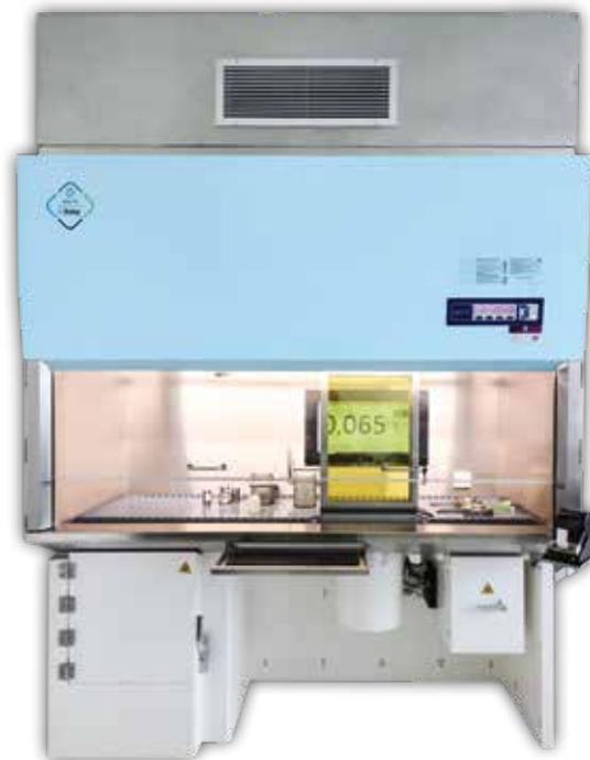
Lead-Shielded Radiopharmaceutical Workstation for Various Applications (PET, SPECT, and 68-Ga, Type EF-N), Ensures increased safety for the user and the product during operations with radioactive substances.
